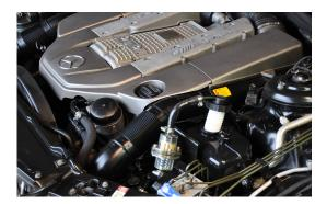
The magnetic filter must be inserted into the black return line leading to the reservoir (black) of the ABC system.
