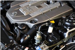
The magnetic filter must be inserted into the black return line that leads to the storage container (black) of the ABC system.
