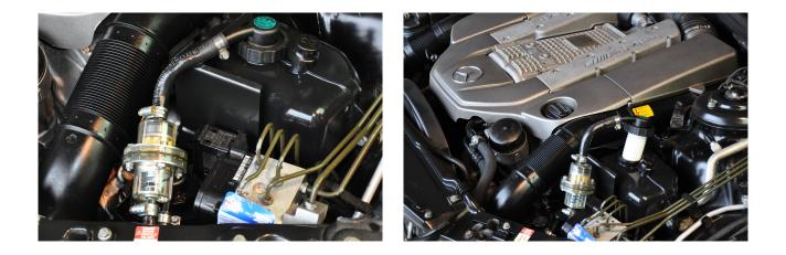
The magnetic filter must be inserted into the black return line that leads to the storage container (black) of the ABC system.
